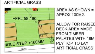
ALLOW FOR RAISED DECK AREA MADE FROM TIMBER PALATES WITH 18MM PLY TOP TO LAY ARTIFICIAL GRASS
